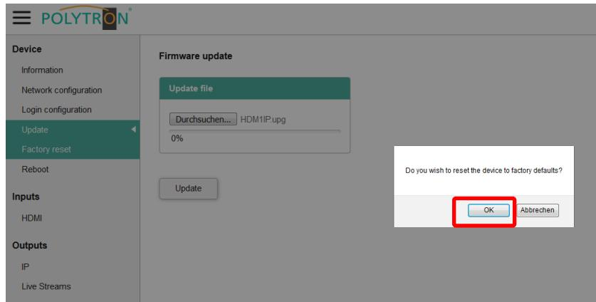
A confirmation message will be displayed on the screen to confirm loading of factory settings. After pressing the button “**OK**“, all settings will be reset to the default values.
