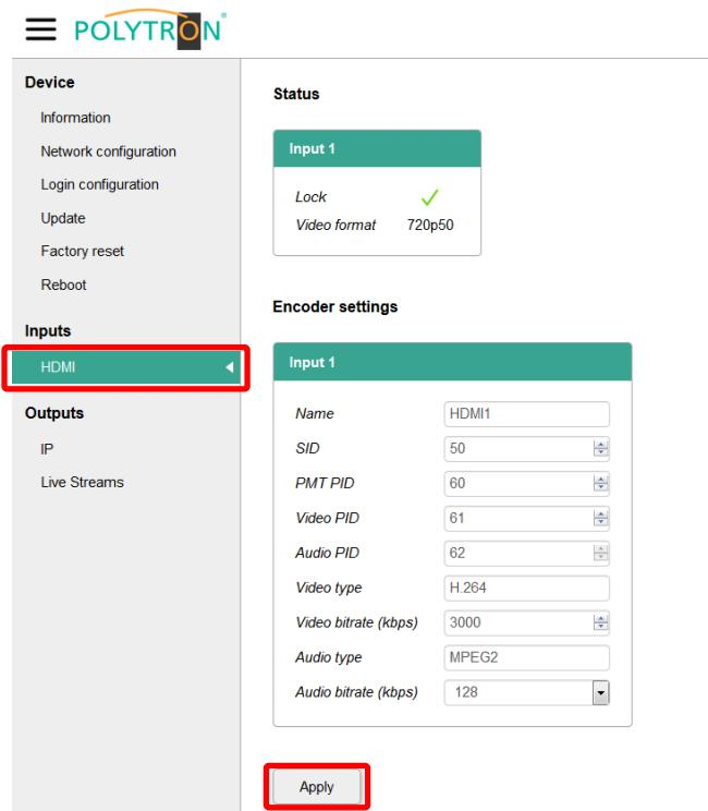
In the monitoring section “**Status**“, the video resolution of the HDMI source and a Lock status for the input will be displayed.
