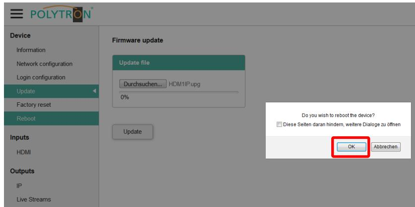
A confirmation message appears on the screen to confirm the restart. After pressing the button “**OK**“, the restart will be done. As soon as the device is ready for operation, the latest active menu will be displayed.
